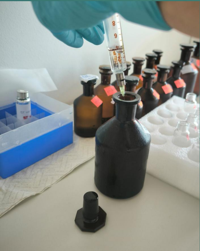
Picture 4. Sample preparation – transfer of samples with a glass syringe
